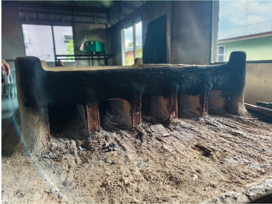
The Belangan used for roasting sago pearls features five fire openings beneath the platform to distribute heat evenly during the cooking process. Photo by the author. Photo by the author.
