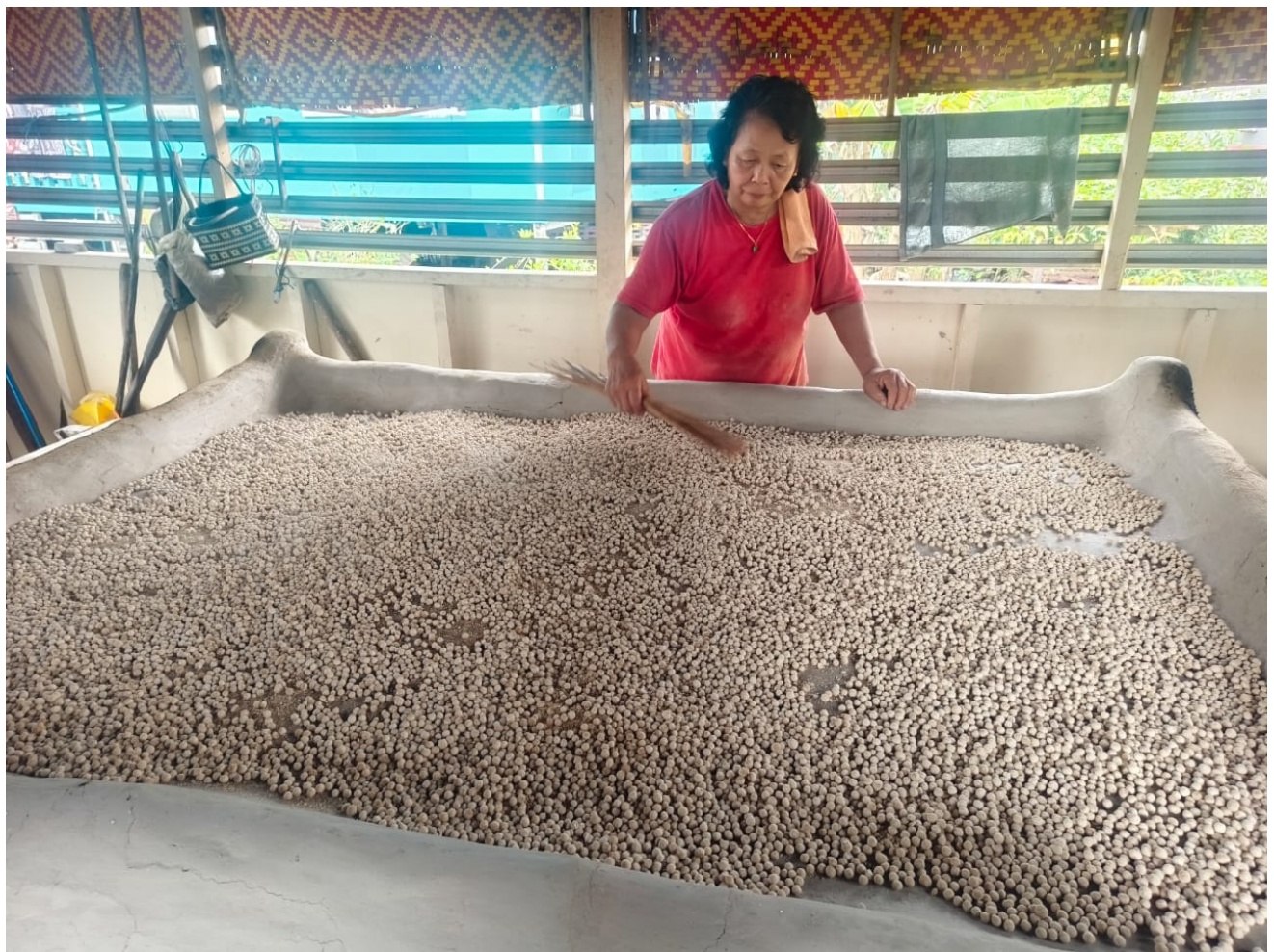
Traditional sago pearl processing site operated by Puan Mary Hubert in Kampung Tellian Tengah. Sago pearls are dried and roasted evenly through controlled heat on the large wood-fired clay stove and constant manual stirring. Photo by the author.
