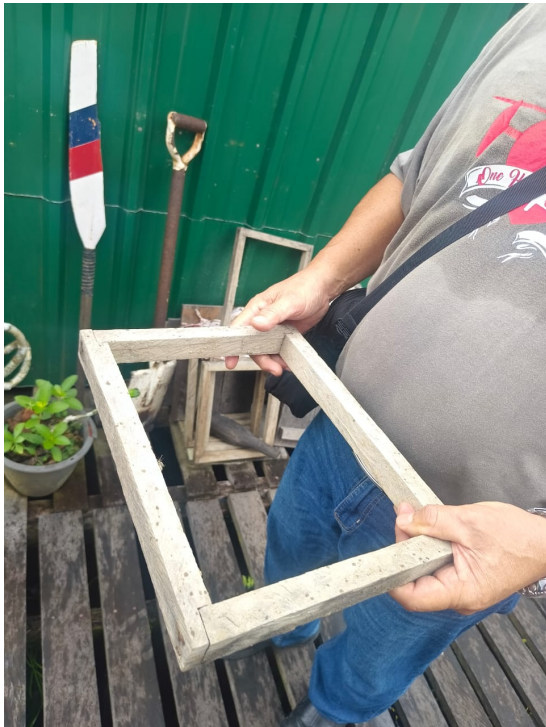
Traditional wooden moulds and clay are used to repair and reinforce the Belangan stove when cracks or damage appear from repeated heating during the roasting of sago pearls. Photo by the author.
