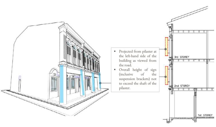
Figure 11 : Signboard Projected From An Upper Storey Pilaster
