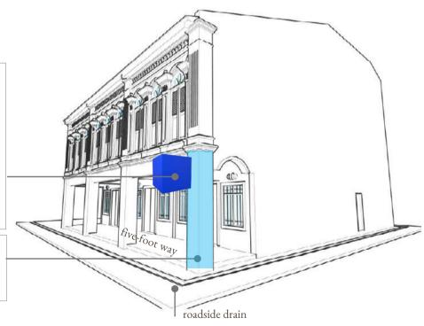
Figure 7: Signs Projected From A Column And Mounted On The Surface Of Column
