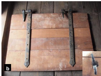
b. Metal strap laid onto cannon door with pre-drilled holes. Custom-made ship nails with split-ends were nailed through metal strap.
