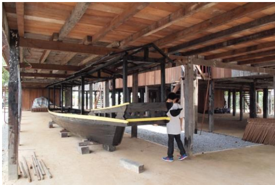
A 34ft long Iban warboat being constructed. Imagine it when it was carrying many warriors!
