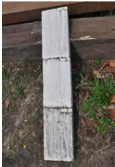
Unsatisfactory results of previous modified lime wash recipes on test panel.
