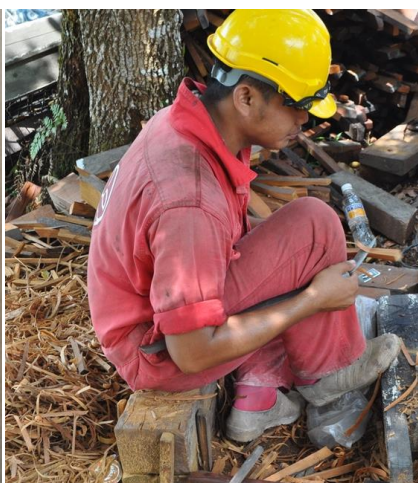
Craftsman anchored his right hand to his leg. The belian piece was dragged across the blade to shape it into a cylindrical dowel.
