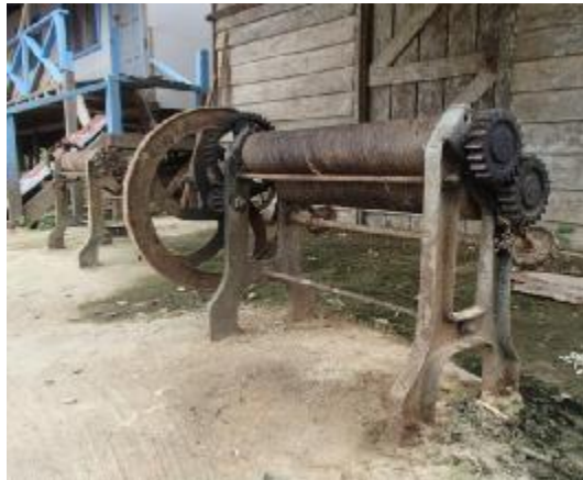
Traditional rubber sheet pressing machine found at the vicinity of the longhouse.
