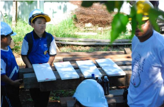
Tan showing test panels of various lime wash ‘recipes’.
