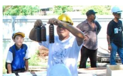
Tan showed darkness of water that corresponds to the length in time for boiling the belian.
