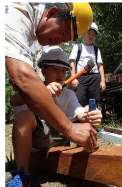
Carpenter Mr Ting guiding a participant to mark the outline of a mortise.
