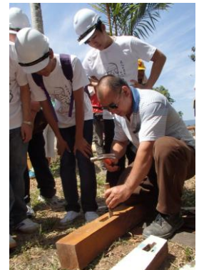
Site Supervisor Mr. Chong Min Chew demonstrating the correct angle at which a chisel should be held.
