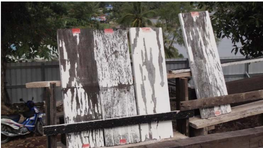
Result of lime wash experiment. The lime wash paint peeled off due to poor adhesion after being exposed to weather for a month.
